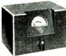
Indicator always shows exact antenna position.
